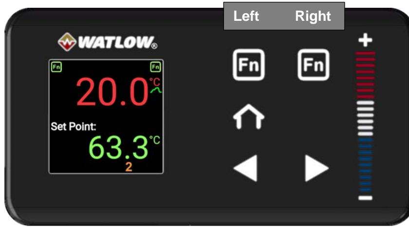
The left function (Fn) button can be used to abort an active profile.
