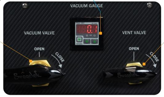
**Vent Valve** controls inlet vent port
